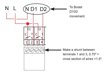
Circuits must be protected by fuse disconnector or circuit breaker 4A maximum. Indicate on the label above the terminal block the location of these protections.
